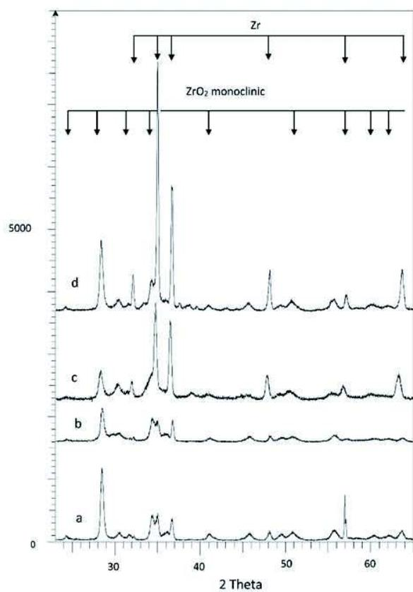
Fig. 2. The grazing incidence X-ray diffraction patterns of (a) initial and enriched with (b) Y, (c) Cr, (d) Al zirconium alloy samples after oxidation in air at 700°C/1000 s following by cooling in water
