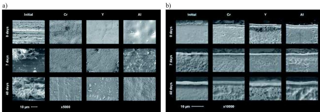
Fig.1. Results of SEM observations of initial, modified and oxidised materials a) surface, b) cross-sections
