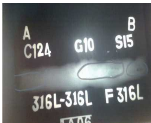
Fig. 7. Copies of X-ray radiographic film for sample No. 07
