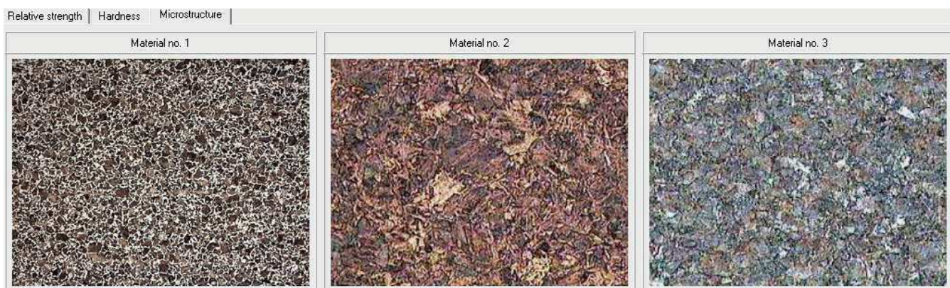
Fig. 5. A comparison of microstructures of three steels 10S20 steel, 25HM steel, 55S2 steel
