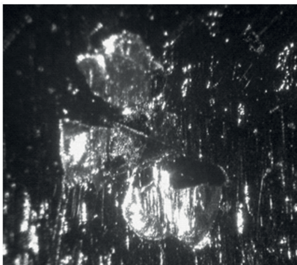
Fig. 5. Indentation results of adhesivity of Ni-P electroless coatings, mag. 35:1, electroless coating + aging at 500°C
