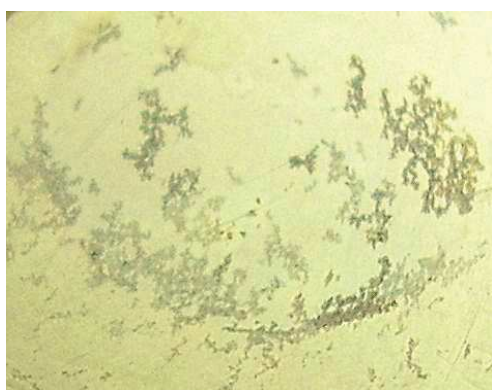
Fig. 5. Appearance of the tested in Na 2 SO 4 solution deformed sample-only blackening is observed
