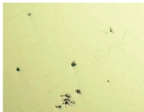
Fig. 4. Appearance of the tested in Na 2 SO 4 solution overaged sample-few pits can be seen
