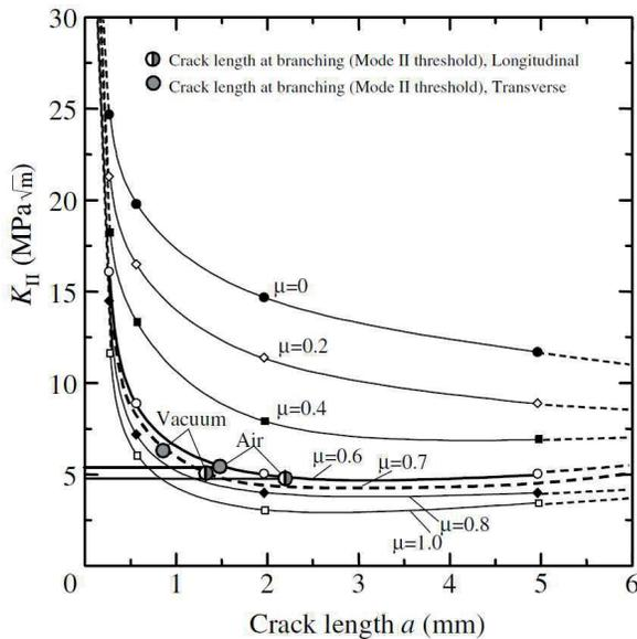
Fig. 9. Relationship between mode II crack length and stress intensity factor for various crack faces friction factor  $\mu$  obtained by FEM [6]
