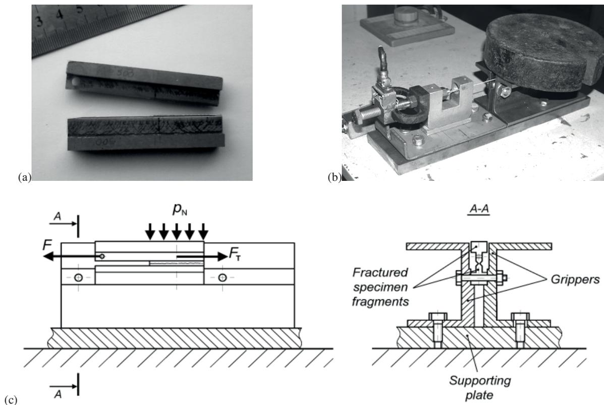
Fig. 2. Fragments of the fractured I-beam specimen (a), device for determining the CFF factor (b), and its working scheme (c)
