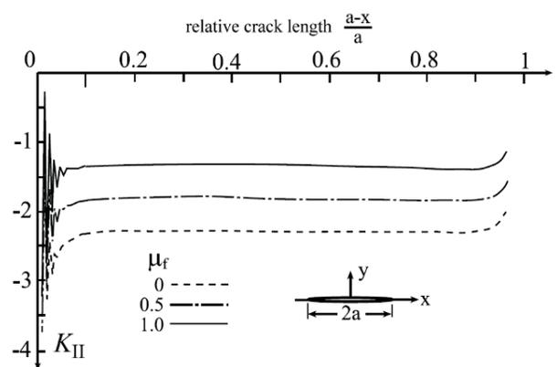
Fig. 8. Normalized stress intensity factor  $K_{II}$  calculated by displaced method for crack friction factor  $\mu_f = 0, 0.5$  and 1 [8]
