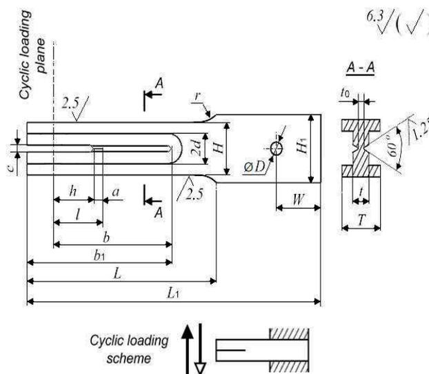
Fig. 1. A specimen for crack growth resistance evaluation of materials under transverse shear
