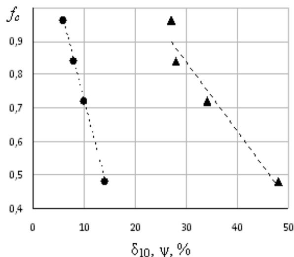
Fig. 5. Influence of elongation (●) and reduction of area (▲) of the 65G steel on CFF factor
