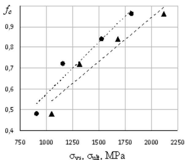
Fig. 4. Influence of yield stress (●) and ultimate stress (▲) of the 65G steel on CFF factor
