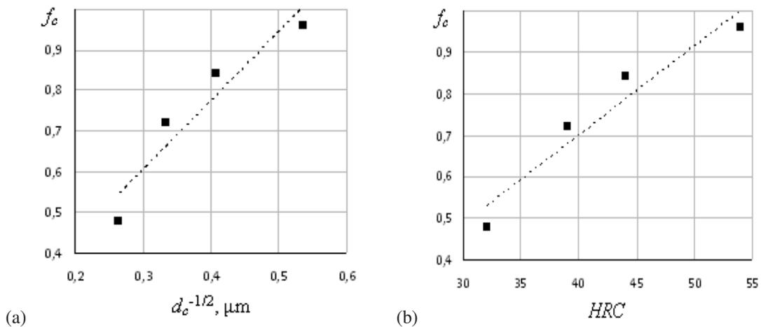
Fig. 6. Influence of cementite groups size in microstructure (a) and hardness (b) of the 65G steel on CFF factor
