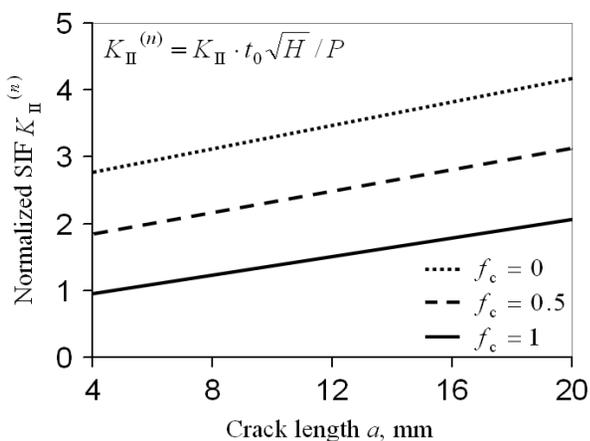
Fig. 10. CFF factor  $f_c$  influence on normalized stress intensity factor  $K_{II}^{(n)}$  for various crack length  $a$  in I-beam specimen
