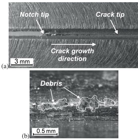
Fig. 7. Mode II fatigue crack in unloaded I-beam specimen (a) made of tempered 65G steel ( $t_{temp} = 500^{\circ}C$ ) and wear debris on the bottom of V-like groove near crack tip (b)
