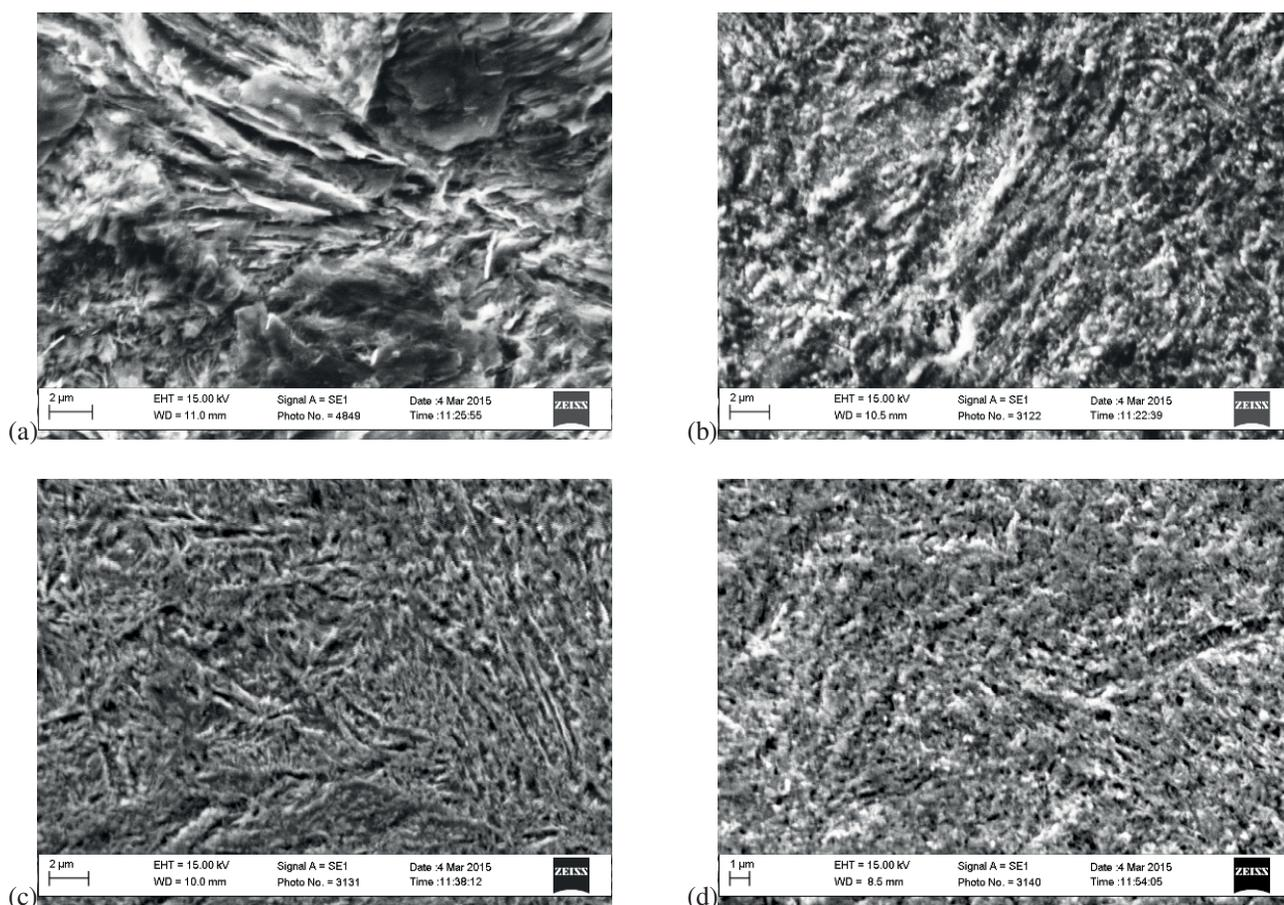
Fig. 3. Microstructure of 65G steel after quenching from 820°C in oil and tempering for 1 h at temperatures: 600°C (a), 500°C (b), 400°C (c), and 300°C (d)
