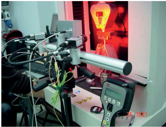
Fig. 2. The testing stand with the Digital Image Correlation system
