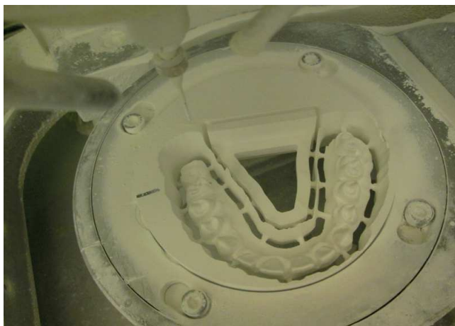
Fig. 5. The milling process of the ceramic suprastructure in the CNC milling machine
